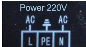
Chart2. Controller power source socket sketch map
